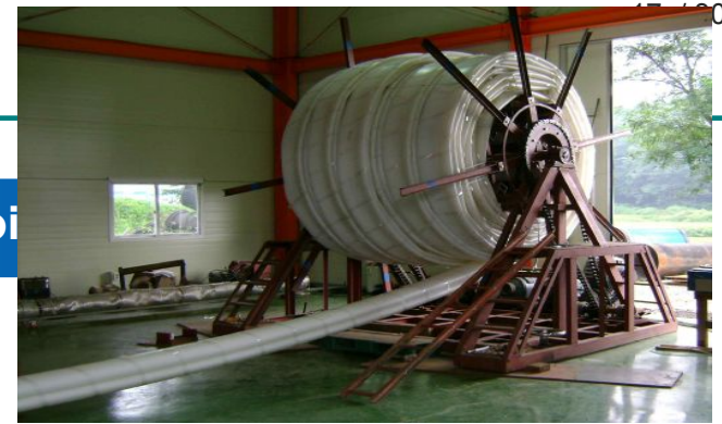
the lining method for rejuvenating the conduit
