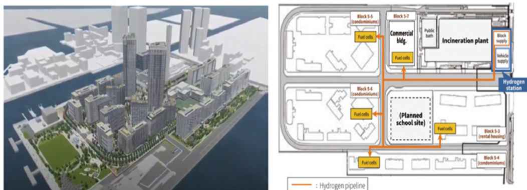
Figure 32: Harumi Flag after completion - bird's eye view and hydrogen supply conceptual schematic.
